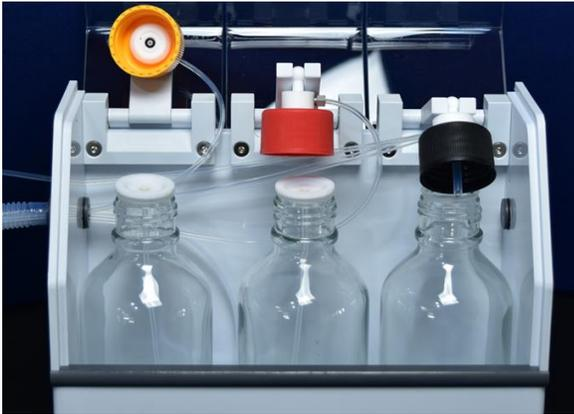
The **Elite Etch** is designed to fit comfortably inside of a fume hood while maintaining all necessary safety features. By using a heat exchange system, waste acid is cooled below 90 C to allow the use of a single waste bottle. The **Elite Etch** uses 3 standard 500 ml bottles which are supplied with the system.
