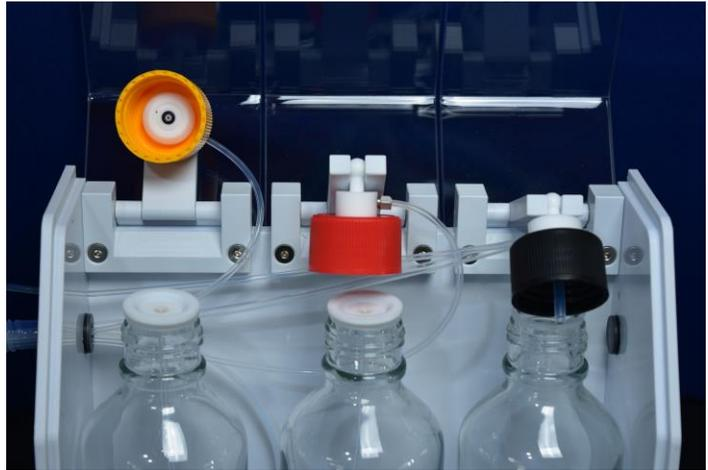
RKD Engineering incorporates double containment for all fluid couplings between the bottle container and the decapsulator. The bottle box assembly and the etcher unit both contain fluid sensors to alert the operator in the event of an acid leak from any of the bottles or internal fittings. The bottle box incorporates a universal pivoting interconnect which allows simple bottle exchange with minimal exposure to residual acid.
