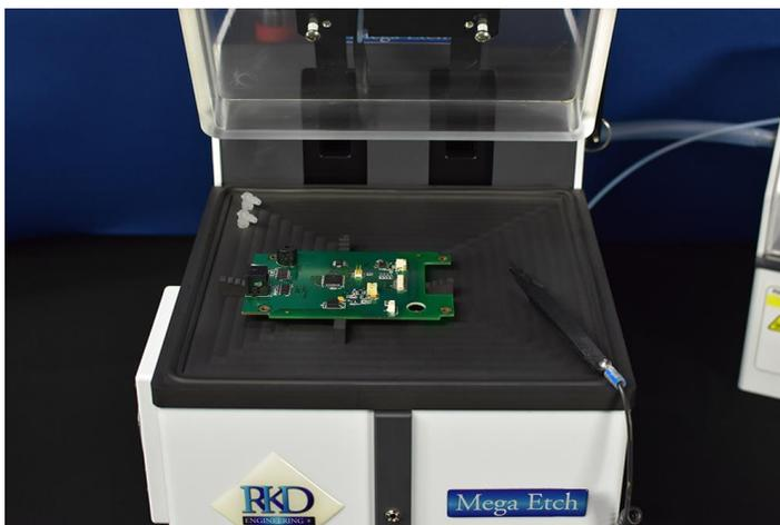
The **Mega Etch** features an acid controller etch head which is machined from premium grade silicon carbide for unsurpassed acid resistance. The etch head is designed to reduce the fuming of any residual acids left on the etch head at the end of the process, both for operator safety and convenient acid disposal.
